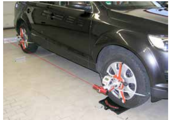
Example of a front axle measurement.
