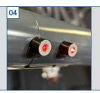
Additional vertical line laser that alternatively enables alignment along the longitudinal axis of the vehicle and thus the increases the number of vehicles that can be tested (e.g. for SUVs).
