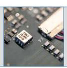
The electronic levelling system compensates for unevenness in the set-up area and is thus an absolute highlight of the MLT 3000. A deviation of only a few millimeters already results in an incorrect assessment of the measurement results. The deviations detected by the position sensor are automatically compensated by the MLT 3000 software, thus avoiding incorrect measurements.
