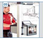
The MLT 3000 2.0 has a robust light collecting box with a large Fresnel lens for simple and quick positioning in relation to the vehicle.
