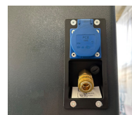
Energy Set with pressured Air and 230 V socket
