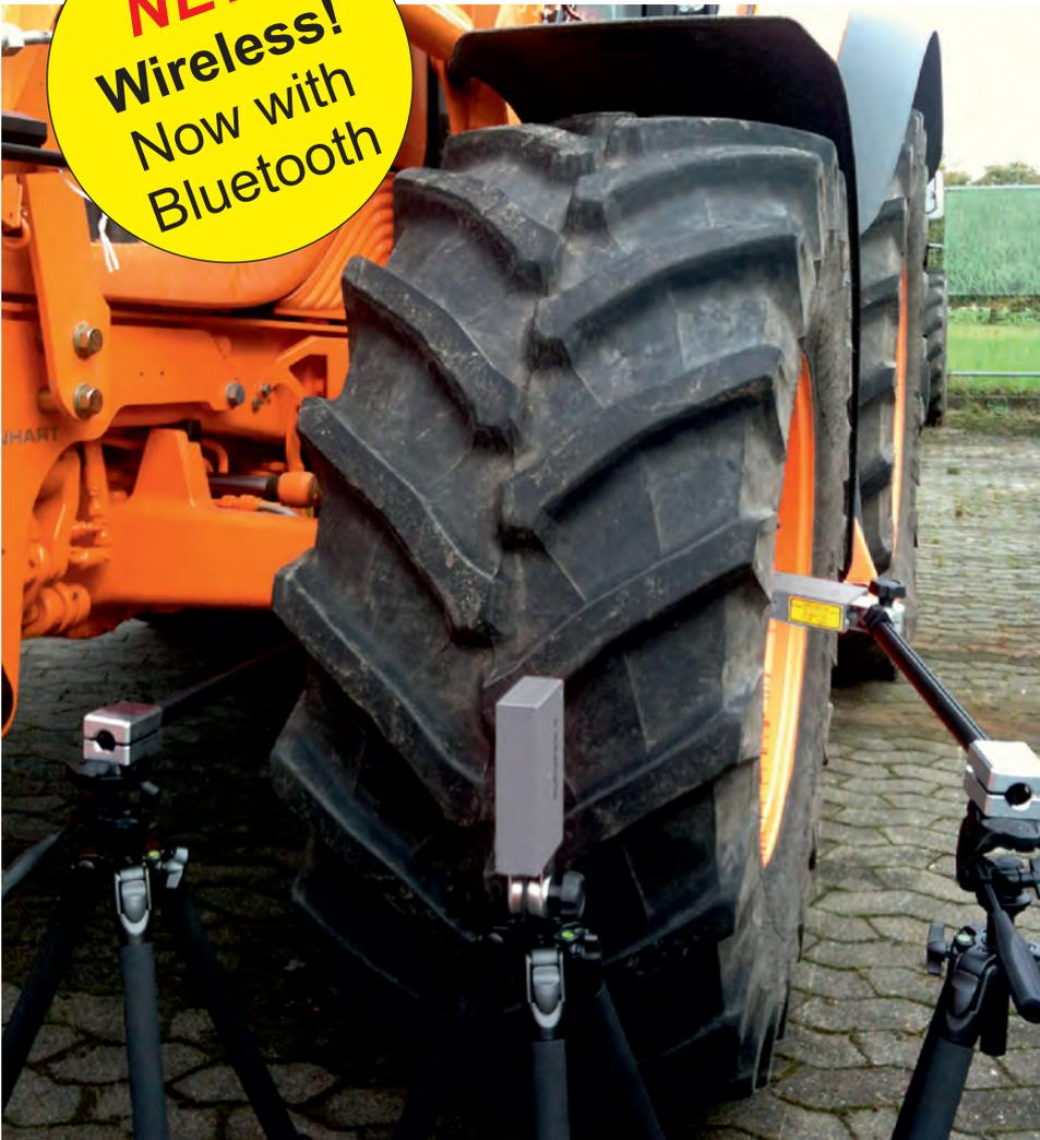
Runout Measurement Device **RPV 1300** for optimisation of the runout of large vehicle tyres.
