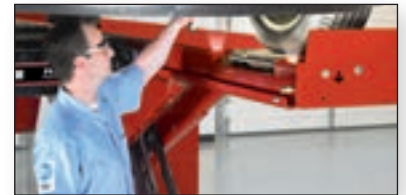
Optional AlignLights system turns on automatically at alignment height
