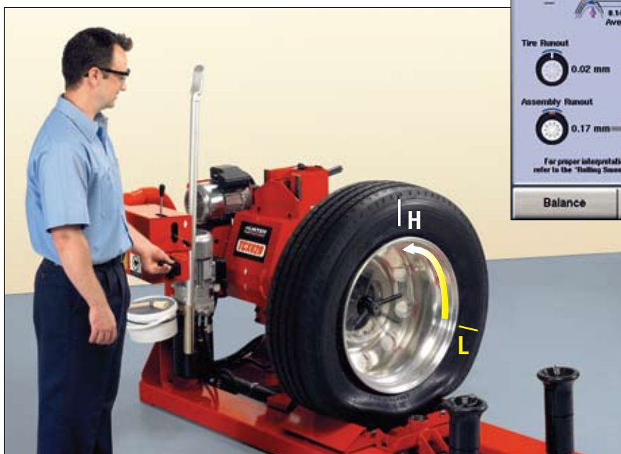
The match-mounting feature on the GSP9600HD tells the technician exactly how to rotate the tire on the rim to minimize vibration.
