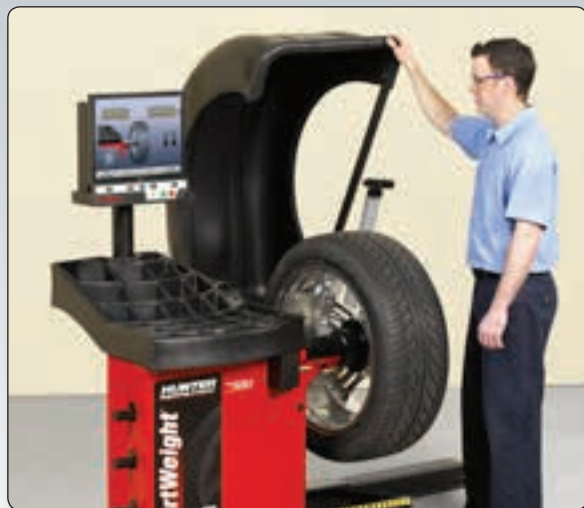
Balance starts when hood is lowered
