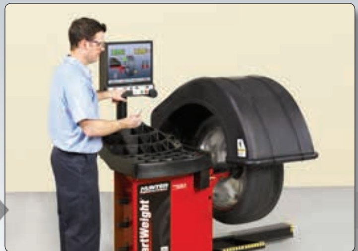
Technician prepares correction weights
