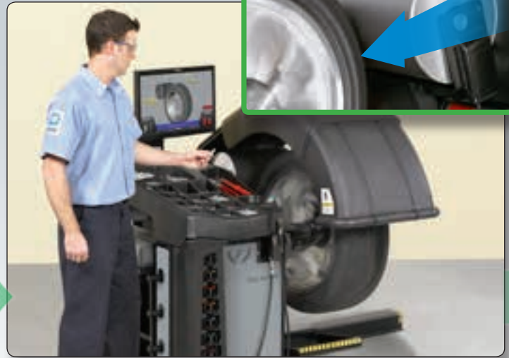
NEW! Load roller measures Road Force while technician prepares correction weights
