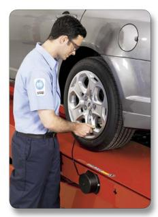
Integrated inflation hoses, located at each wheel position, retract when not in use to keep the work area clear.
