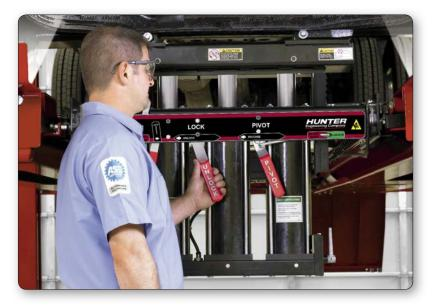
**9,000-lb. Capacity, Triple Composite Cylinder Jack: 133-84-1**Ideal for use with RX16, L441 and L444
