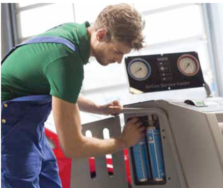
Standard on ASC 1000 G units: humidity free storage and feeding system for fresh oil and UV additive
