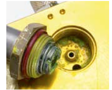
Sealant contamination in the A/C service unit without the use of the Recycle Guard
