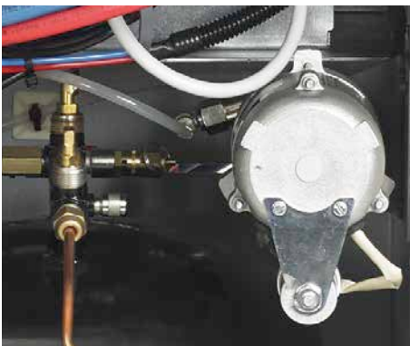
Integrated fluid pump: For charging high-volume A/C systems
