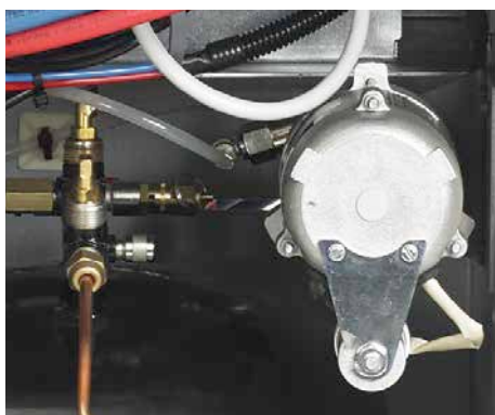
Integrated fluid pump: For charging high-volume A/C systems
